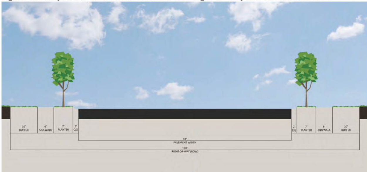
Figure 4.7: Major Arterial Cross-Section 128 Feet Right-of-Way and 78 Feet Pavement
