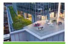
**Green Roofs: Vegetated** rooftops provide insulation to buildings, reduce reflection and heat radiation, reduce stormwater runoff to adjacent surfaces, and can offer building residents a place to relax.
